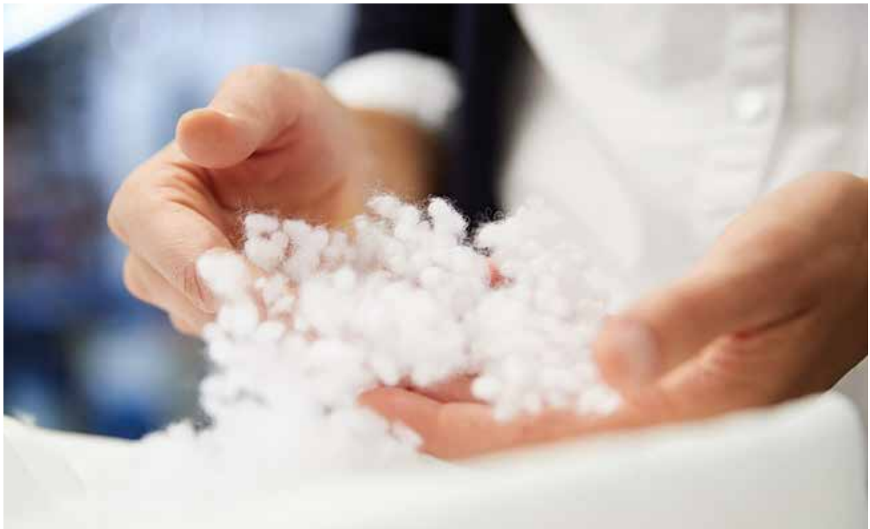
Comfortemp Fiberball is a padding made from linked fiber balls, making it suitable as thermal padding in sportswear and functional textiles.
