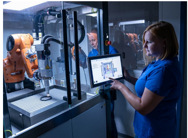
Freudenberg Technology Innovation employees working with the new atmospheric-pressure plasma jet device.
