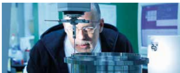
After production, the metal housing in the mechanical seals are tested using 3D monitoring.
