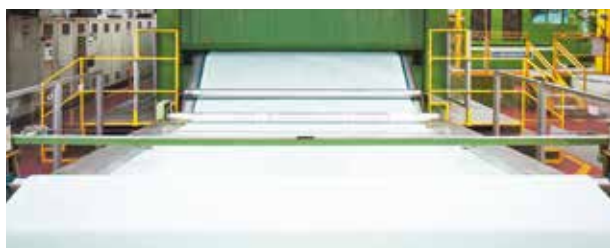
Recycled polyester is used to manufacture nonwovens used in roof seals as well as acoustic and thermal insulation.
