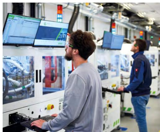
Fuel cell test bench at Freudenberg Sealing Technologies, 2019
