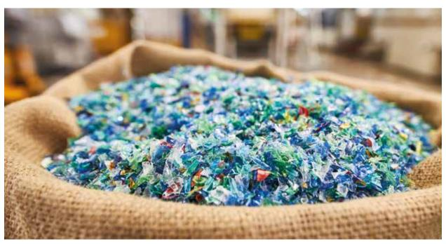
$PET\ granulate\ made\ from\ recycled\ source\ material\ is\ used\ in\ the\ Vileda\ and\ O-Cedar\ brands\ from\ Freudenberg\ Home\ and\ Cleaning\ Solutions.$
