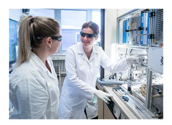
Two Freudenberg Technology Innovation employees working with a coating unit that uses UV polymerization. They are wearing special UV protective glasses.
