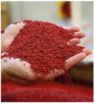
One example of a sustainable solution is employing used and recycled plastic. Recycled polypropylene pellets are transformed into red components for the Vileda brand of the Freudenberg Home and Cleaning Solutions Business Group. Here the focus is on objectives 12 and 13 on the list of Sustainable Development Goals.
